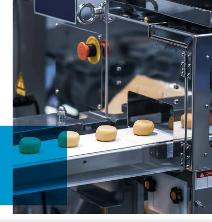
During cookie production, many bakeries use an automated cutting knife to portion dough onto a conveyor. Without proper lubrication, the cutting knife and conveyor belt become sticky with built-up dough, forcing workers to stop the process so they can clean the equipment manually. This leads to excess labor hours and lost productivity.
