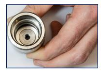
Install the swirl into the carrier, swirl side toward orifice disc. (TIP: hold the carrier at a 45 degree angle with the 2 lugs at 12 o'clock. Align the flat side of the swirl at 12 o'clock. The swirl will drop into place).
