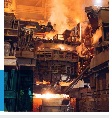
Cooling of exhaust gases from the Electric Arc Furnace (EAF) is critical to controlling temperatures of the gas in the ductwork as it enters the baghouse to prevent a fire. Air atomizing nozzles are ideal for cooling the gases because they produce very fine droplets, but air consumption can be high and costly if the proper nozzle is not selected.
