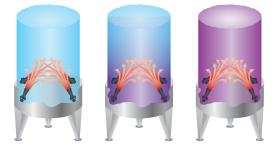
cause batches to be ruined. Eductor nozzles, like the BETE TurboMix<sup>®</sup>, reduce the settling of suspended particles, improve circulation, and maintain uniform liquid characteristics. They offer a lightweight, inexpensive alternative to mechanical mixing methods.
