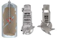
internal gears on the body to rotate sets of high impact jet nozzles through an efficient 2-axis orbital pattern, providing complete 360° coverage. The jet pattern nozzles utilized on these assemblies provide significantly more impact and impingement force than other styles of tank cleaning nozzles, making them ideal for hard to clean residues and larger vessels.
