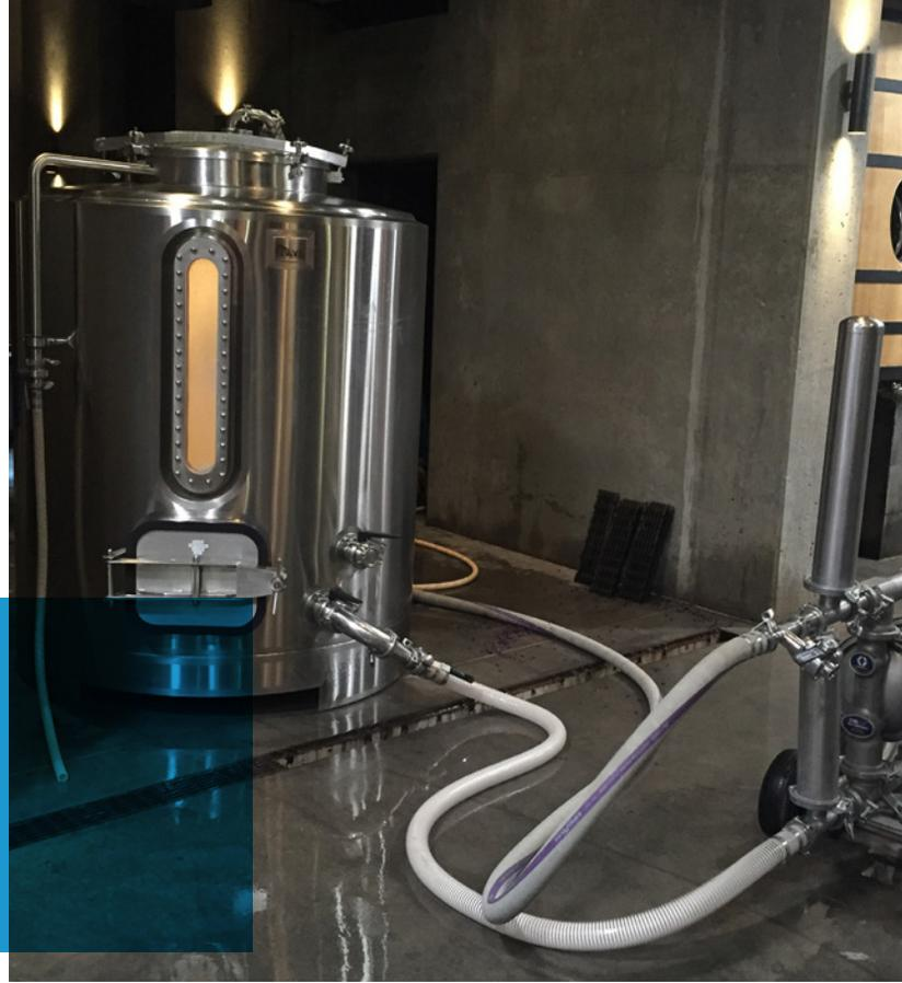
Even with a preliminary rinse before the cleaning process, leftover grape debris in the fermentation tanks such as seeds, stems, and skins remain.
