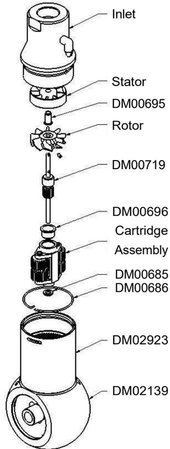
Figure 13: Body shell and inlet casing
