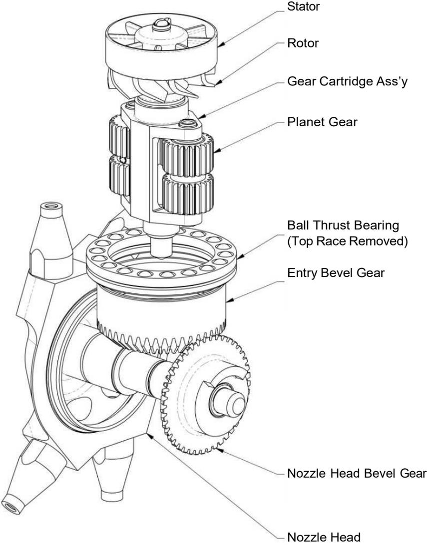
Figure 2: Orbitor tank washing machine with housings removed.
