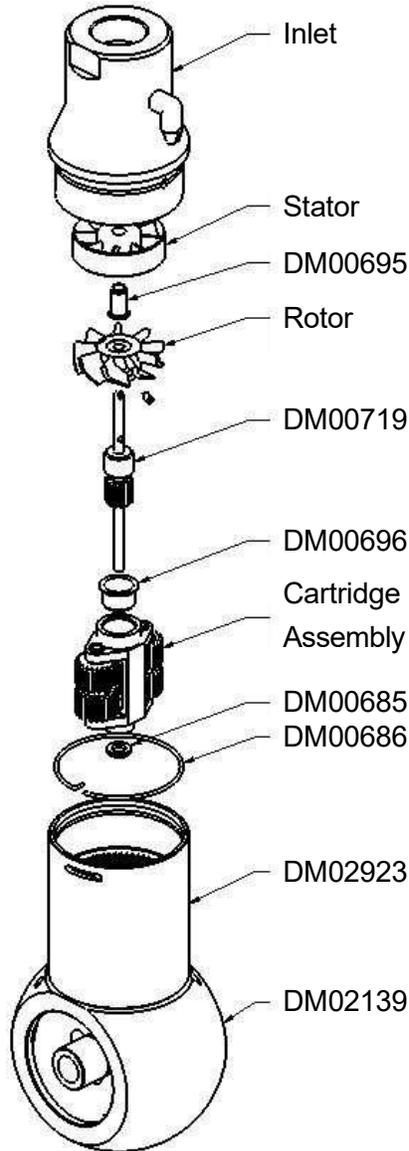
1. Hold machine by inlet casing at the bottom and turn the body shell (DM02140) counter-clockwise by hand, or alternatively with a strap wrench if tight.
