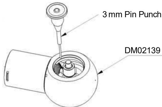
Figure 9: Pin removal
