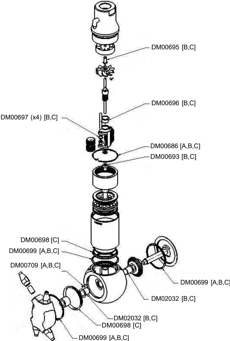
Figure 19: Rebuild kit components. Letters in brackets are the kits in which that component is included.
