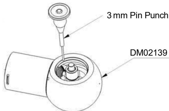
Figure 12: Pin insertion
