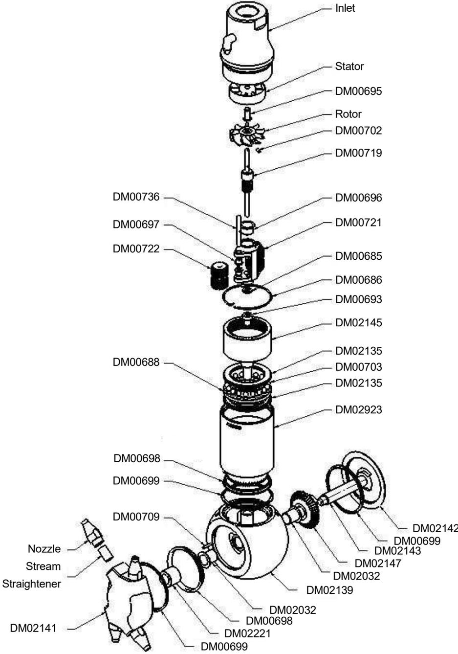
Figure 18: Exploded view of the Orbitor
