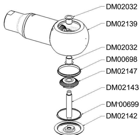
Figure 14: Back plate reassembly
