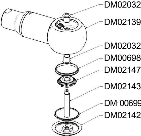
Figure 5: Back plate disassembly
