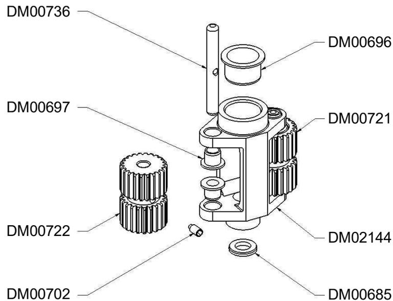
Figure 8: Gear cartridge subassembly
