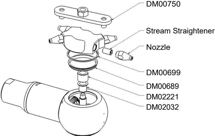
Figure 15: Nozzle head reassembly
