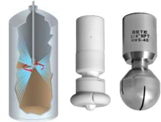
reaction force of the spray media to drive the rotation of the nozzle head. These provide complete 360° coverage and efficient cleaning through impact and repetition. Rotating nozzles ensure a significant increase in tank washing efficiency over static spray balls, saving time and money by reducing water and cleaning agent consumption while decreasing downtime.
